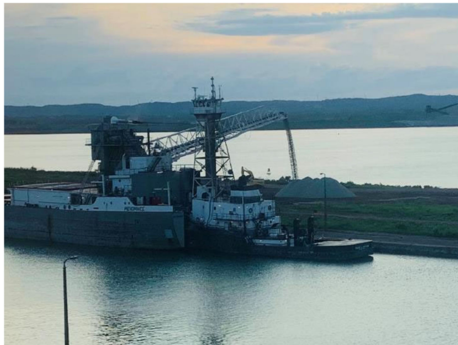
Menominee Unloading Aggregate on Northwest Pier in support of Upstream Channel Deepening Contract
